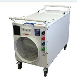
Efficient, versatile and reliable, the I60KRH portable electric resistance heater produces clean, dry, safe heat offering an ideal environment for a variety of special event, emergency, disaster or construction applications. The duct-in/duct-out solution adds versatility by allowing you to switch between fan only, 20kw, 40kw and 60kw of heating. The unit comes with unit mounted controls. Power connections are CamLock connectors.
